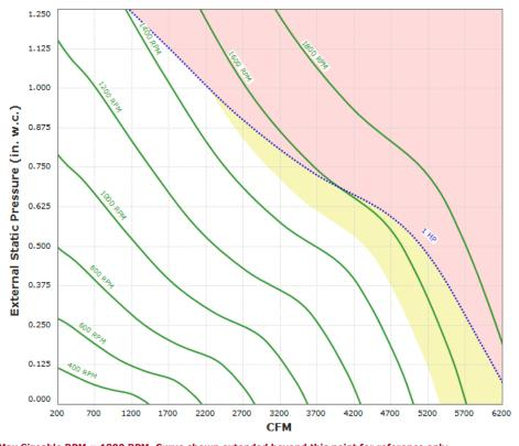
Max Sizeable RPM = 1800 RPM. Curve shown extended beyond this point for reference only. Motor M055PWCUK0315-ECM-50-115 has an rpm range of 300 to 1800. Motor M055PWCUK0315-ECM-50-230 has an rpm range of 300 to 1800. Motor M055PWCUK0315-ECM-60-115 has an rpm range of 300 to 1800. Motor M055PWCUK0315-ECM-60-230 has an rpm range of 300 to 1800.
